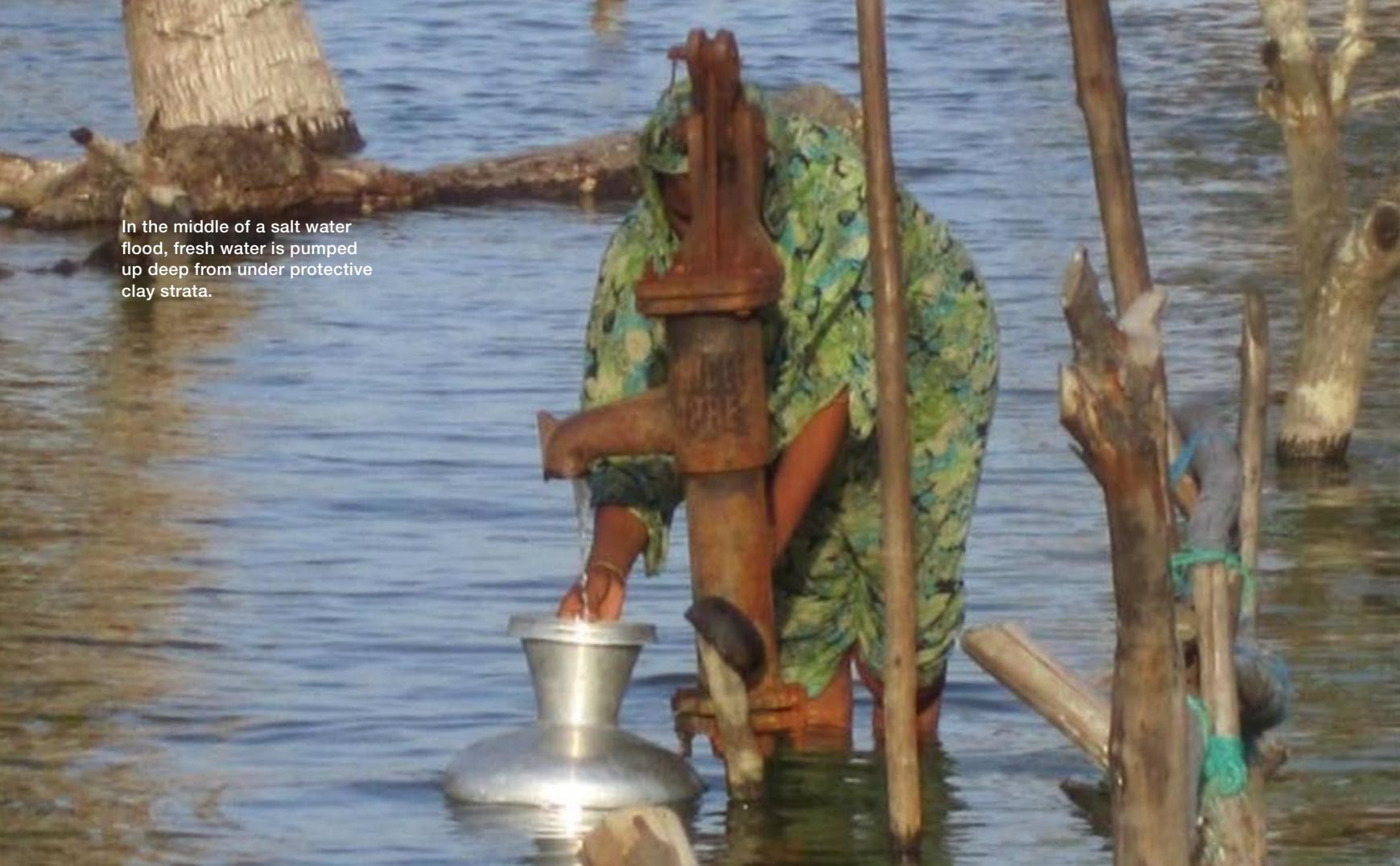
In the middle of a salt water flood, fresh water is pumped up deep from under protective clay strata.
